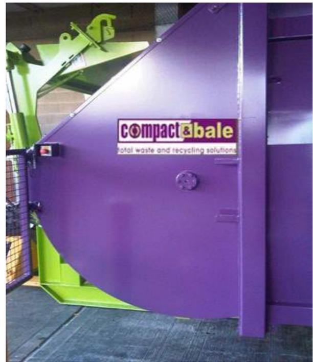
Safety guarding is simple yet effective using a spring assisted lid (rather than an auto opening system that has often damaged, moving parts and requires full height guarding that hinders operation and loading) together with a pair of manual interlock mesh safety gates and a two-hand user control to keep your operator safe while completely removing the on-going cost of regularly broken magnetic interlock switches, latches, catches and hinges from repeatedly slammed gates.
